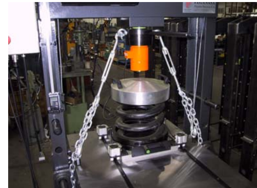
Special press to test accurately the strength of the springs of a train suspension
