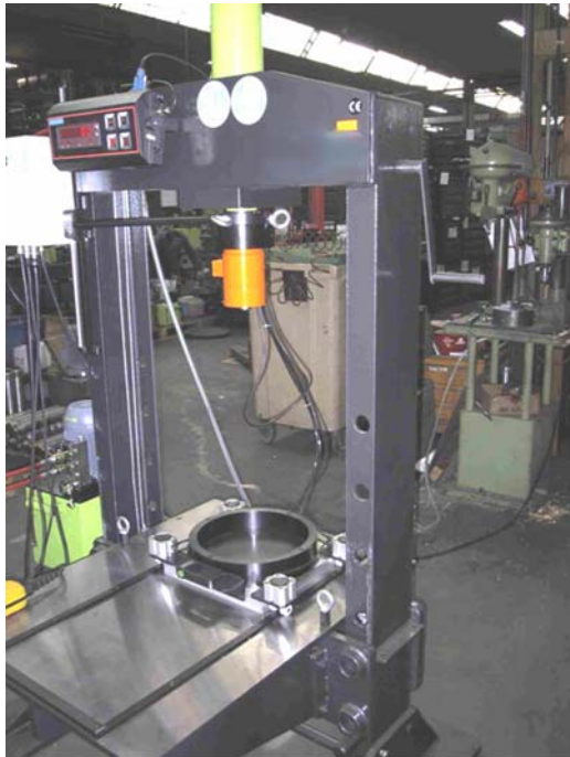
Special press to test accurately the strength of the springs of a train suspension
